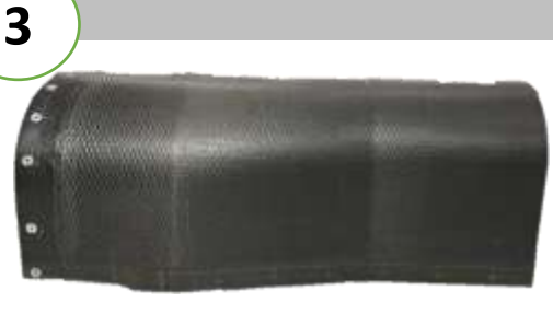
ITSC, LOX, LH2 WIRE TUNNEL & BOTTOM PLATE ASSEMBLY
