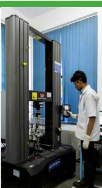
100KN – Universal Testing Machine (UTM).
